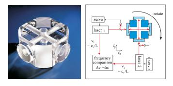
FIG. 1: Left: High-finesse fused silica resonators used in this experiment. Right: Basic principle of the experiment. The frequencies of two lasers, each stabilized to one of two orthogonal cavities, are compared during active rotation of the setup. (Photograph by E. Fesseler)
