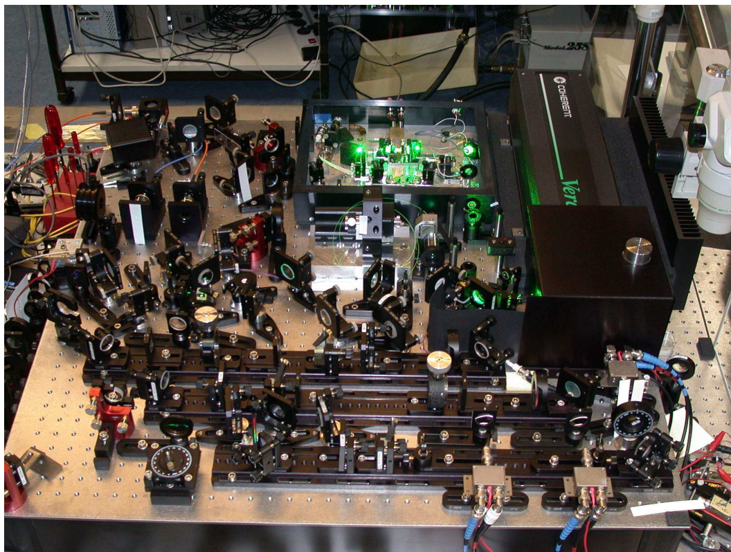
Figure 6.12: Photograph of the Ti:Sapphire femtosecond laser frequency comb setup.
