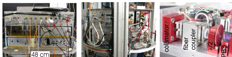
Figure 2.10: Mechanical mount of the laser system. Optic (left) and electronic (middle) racks have the standard width of 19". Mounts for optics with the beam height of 20 mm (right).
