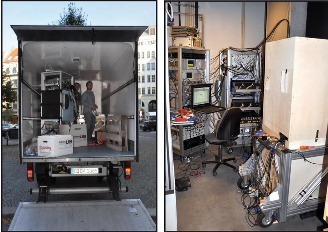
**Figure 5.10:** Transport of gravimeter from assembly laboratory to first measurement site in Berlin-Adlershof. Left: loading the gravimeter onto the truck, right: gravimeter during measurement at Berlin-Adlershof site (from left to right: electronics/control rack, laser rack, physics package).
