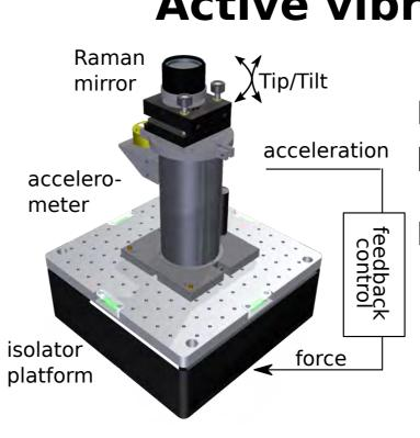
Modified minusK vibration isolation platform with active feedback control
