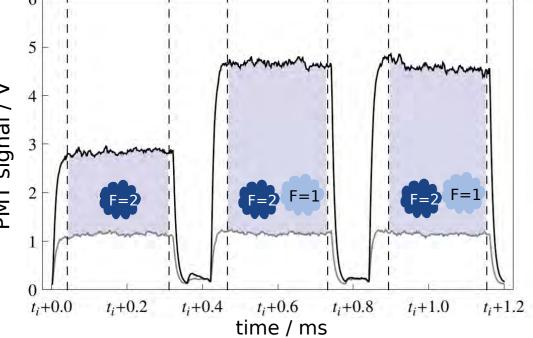
Detection pulses with intermediate repumper light
