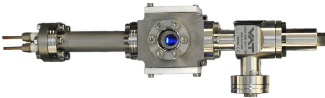
Figure 1: Currently employed spectroscopy cell with a simple strontium source
