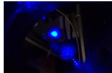
**Left: Currently employed spectroscopy cell with a simple strontium source. Right: A cold cloud of strontium atoms, laser cooled in a magneto optical trap. This will be the starting point of our new setup.**
