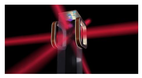
Schematic of a laser-cooled atomic ensemble experiment. The student will work with a similar system in our labs (photo from NASA).
