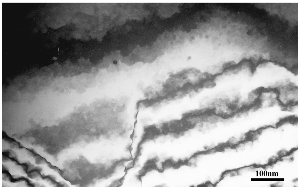
Figure 42. BF-TEM image of SiC (111) demonstrating partial success in creating atomically flat surfaces. Recorded on JEOL4000 at 400kV and a magnification of 60000 \times .
