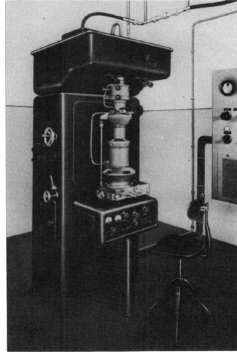
FIG. 11. First serially produced electron microscope, by Siemens. General view (von Borries and Ruska, 1939).
