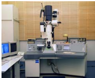
Zeiss 912: 200kV, in-column filter
