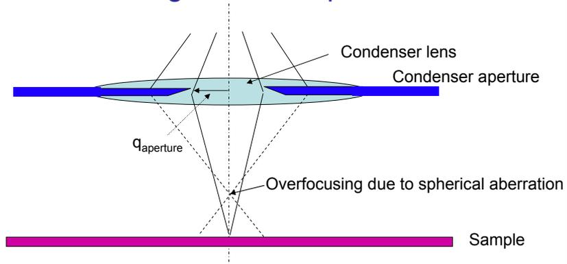
The probe is an image of the electron source. The probe size depends therefore on the same parameters as the resolution in a TEM image.
