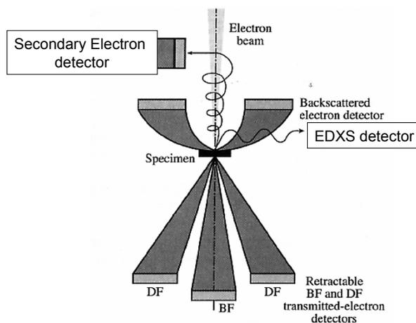
Normally, a STEM is equipped with several detectors which can collect their respective signals simultaneously. The BF detector may usually be replaced by an electron energy loss spectrometer (EELS).
