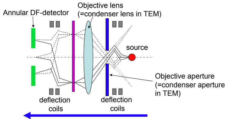
Note: The analogue technique to ADF-STEM in the TEM is hollow-cone dark-field (HC-DF) TEM, in which the illumination angle is rotated about the optic axis during the exposure of the image.
