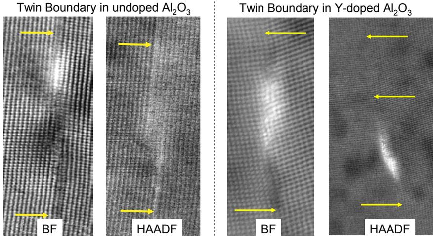
HAADF-STEM is much less sensitive to local diffraction conditions than BF-STEM. Because of its sensitivity mainly to the atomic number, it is also called Z-contrast STEM.
