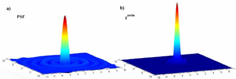
2-dimensional impulse response function ( $PSF(\vec{r})$ ) and STEM probe function  $I^{probe}(\vec{r})$  for the same microscope parameters ( $E = 200\text{kV}$ ,  $C_s = 0.7\text{mm}$ ,  $\alpha = 12.5\text{mrad}$ ,  $df = -513\text{\AA}$ ). The scale in x- and y-direction is in  $\text{\AA}$ .
