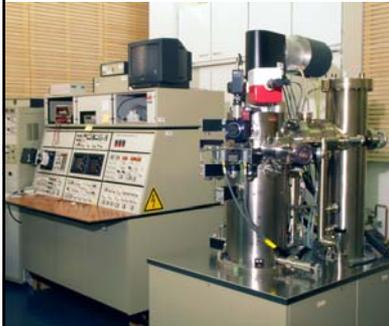
Heavy pumps needed for gun-UHV must be located at the bottom for stability reasons.
