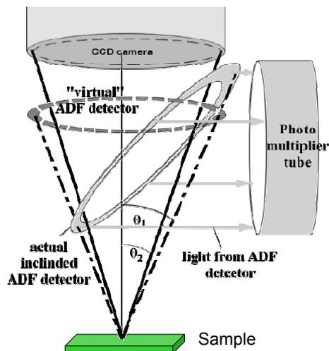
Perfect setup for Ptychography, a holographic method, which promises diffraction-limited resolution (i.e.  $\ll 1\text{\AA}$ ). ...
