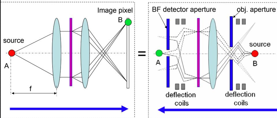
The scanning of the electron beam in a Scanning Transmission Electron Microscope (**STEM**) corresponds to the different pixel positions of a TEM image detector, if the range of scattering angles accepted by the bright-field detector equals the reciprocal-space source size. (Note: the objective pre-field in the TEM performs a Fourier transform)
