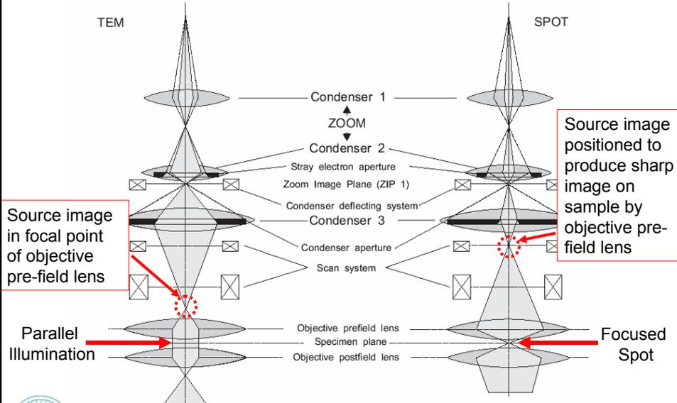
Example: 3-condensor system of a Zeiss Libra 200
