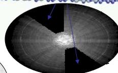
(Here only part of the ADF detector is shown in the diffraction patterns, in order to show its size)
