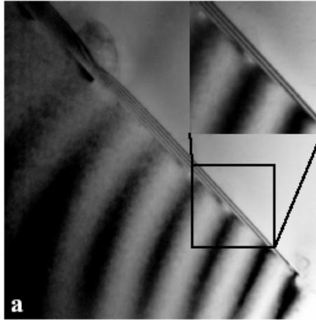
Thickness fringes in a BF image of a grain that is in, or close to a zone axis and shows therefore strong dynamical effects.
