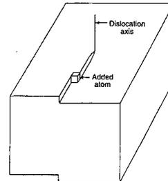
Spiral crystal growth around the core of a screw dislocation
