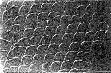
Two sets of dislocations are visible; the stacking faults are invisible.
