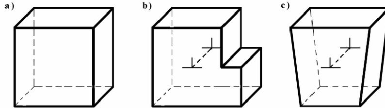
Operations producing pure edge dislocations a) perfect crystal cube b) shear: the horizontal lattice constant of the top part of the crystal due to shear stress differs from the one on the bottom. Misfit dislocations account for the displacement on the atomic level. c) dilatation: edge dislocations moving through the perfect crystal structure account for material shift in ductile processes.
