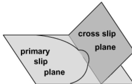
The screw part of a dislocation loop may deviate in a cross slip plane. The dislocation Burgers vector is along the intersection of the primary and the cross slip planes.
