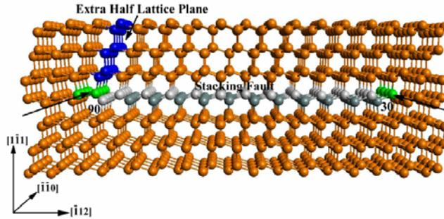
Dissociated 60° glide-set dislocation. A stacking fault (SF) ribbon (plane of gray and white atoms) is bound by the two partials. The cores (green) of the 30° and the 90° partial are reconstructed. The extra half plane at the 90° partial is indicated by the blue atoms.
