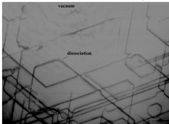
BF image of dislocations in Si(111). The dissociation of dislocations into partials can be seen very clearly. The very weak contrast features concentric around the small area of vacuum at the top of the image are Pendellösung fringes.
