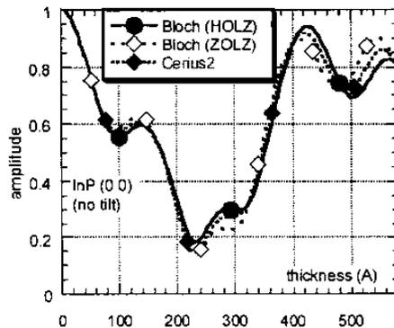
Plot of the (dynamical) intensity of the central beam of a diffraction pattern of InP (100) as a function of specimen thickness.
