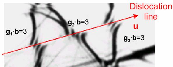
If the dislocation line intersects with only one HOLZ line, the sample (or illumination) can be shifted to make it intersect with another HOLZ line.
