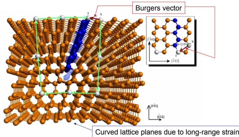
Burgers circuit in diamond cubic structure containing a dislocation running into the plane of the paper as indicated by the round (blue) arrow. The length and direction of the Burgers vector is the difference between the points S and F. The inset shows a portion of the top plane, showing that the Burgers vector  $b = \frac{1}{2}[10\bar{1}]$  is not in the plane of the paper, but at a 60° angle with respect to the dislocation line.
