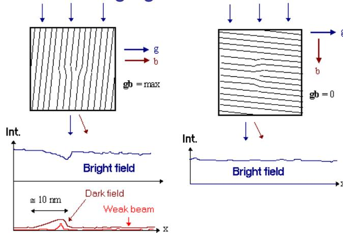
A Burgers vector of  $\mathbf{b}$  of a dislocation produces a local shift in lattice constant in the direction  $\mathbf{b}$ . If a 2-beam condition for reflection  $\mathbf{g}$  is set up, contrast of dislocations whose Burgers vector is parallel to  $\mathbf{g}$  is maximized.
