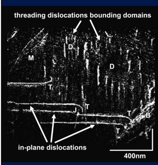
GaN film showing walls of threading dislocations surrounding domains (D), a dislocation bundle (B) associated with a crack, and threading dislocations that turn over at T to become in-plane dislocations and terminate at the specimen surface. Each turn over T occurs at a different height in the film, and one has interacted with a threading dislocation, causing a jog (J). Dislocations of mixed character (M) are also visible.
