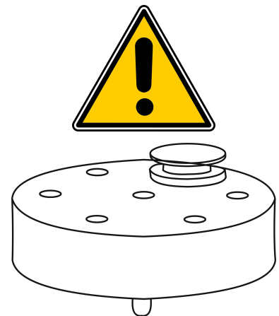
Figure 3.1: A multi-stub holder for seven stubs, with one stub inserted; the latter supports the specimen.
